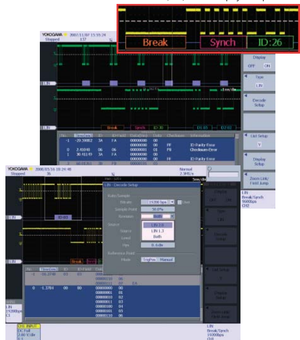
Figure.13 LIN revision 1.3 and 2.0 simultaneous decode, analysis display example
