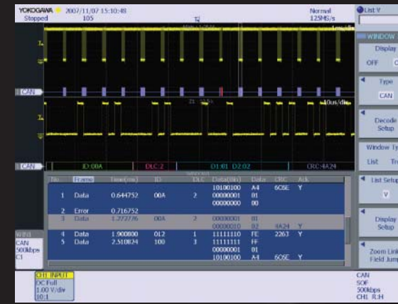
Figure.7 CAN waveform, list, decode display example
